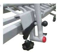
A Ensure either end of the side rail is less than 60 mm or more than 318 mm from the bed end to minimise risk of entrapment.
